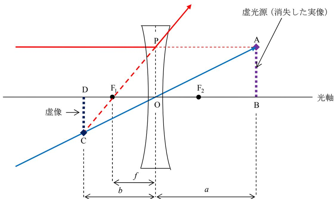
$$\triangle ABO \sim \triangle CDO \text{ より, } \frac{AB}{CD} = \frac{BO}{DO} = \frac{a}{b} \quad \dots \textcircled{12}$$
