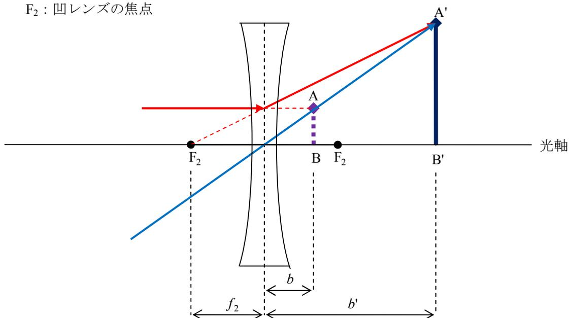
$$f = \frac{f_1 f_2}{f_1 + f_2} \text{ より, } f_2(f_1 - f) = f_1 f$$
