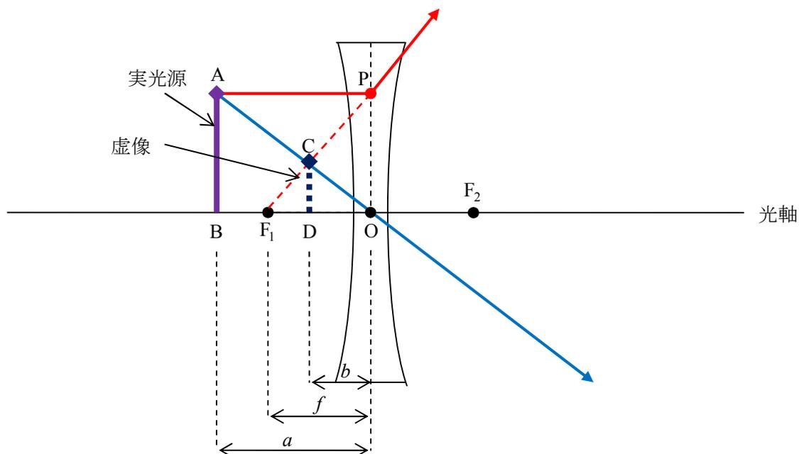
$$\triangle ABO \sim \triangle CDO \text{ より, } \frac{AB}{CD} = \frac{BO}{DO} = \frac{a}{b} \quad \dots \textcircled{9}$$
