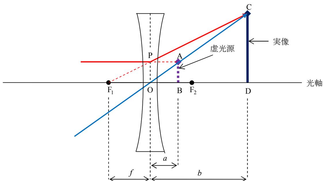
$$\triangle ABO \sim \triangle CDO \text{ より, } \frac{AB}{CD} = \frac{BO}{DO} = \frac{a}{b} \quad \dots \textcircled{15}$$
